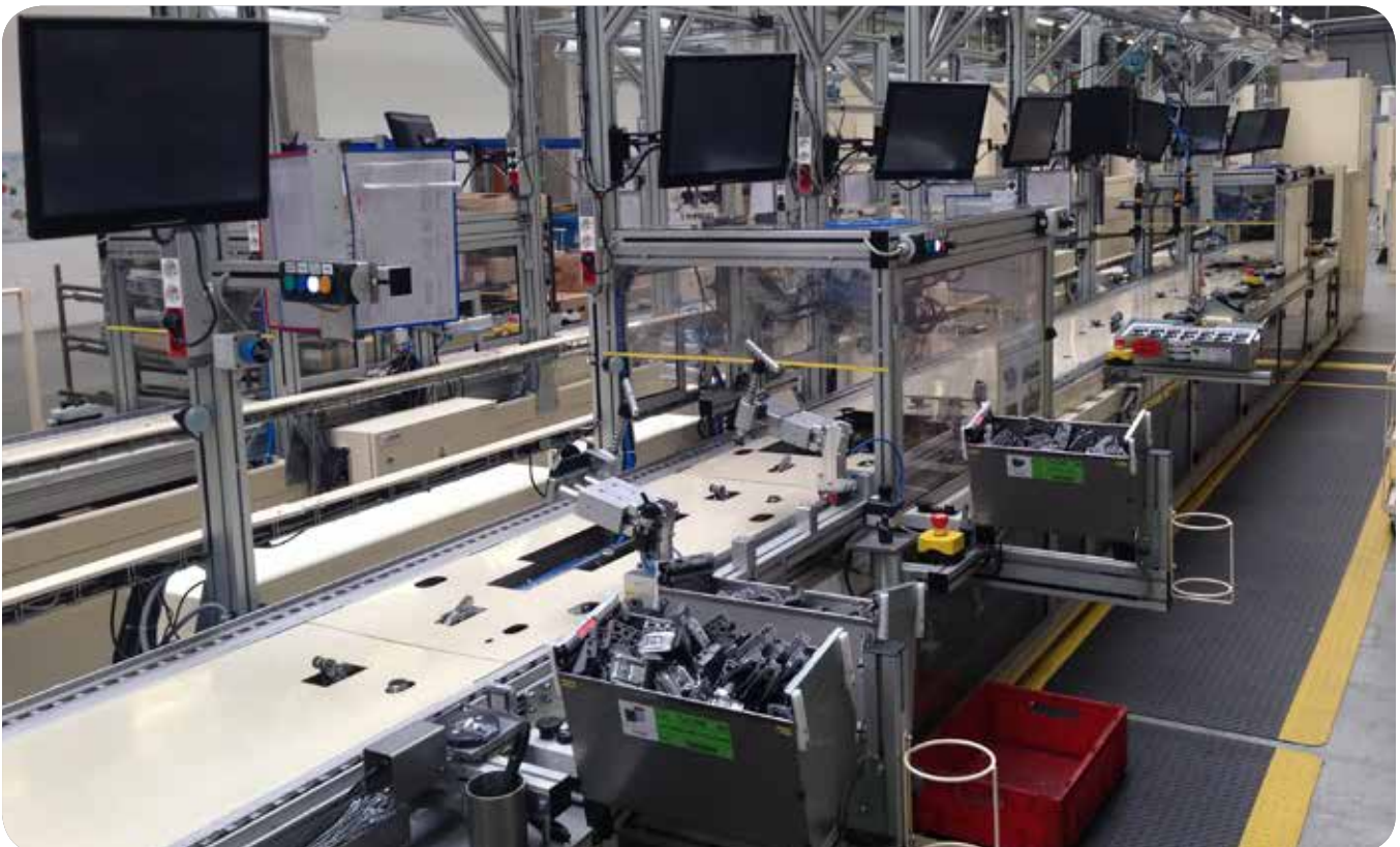
The assembly line is designed to meet demanding production capacities and targets and is capable of building 850 car sets per day
